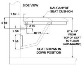
Ensure that the appropriate finished seat height line is at the desired height and is level.
