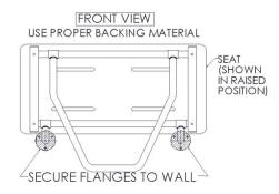
Holding the seat assembly in an upright and raised position against the wall, tightly secure the two mounting flanges to the wall **AND INTO PROPER BACKING MATERIAL**, using mounting hardware suitable for your specific mounting application.
